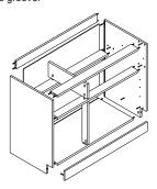
**Step 3:** Attach the Undermount soft-close slides onto the side panels using the pre-drilled holes and the nickel round head screws.
