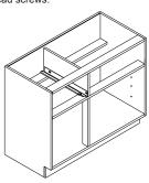
**Step 4:** Assemble the drawers and install the drawer front connector on the underside of the bottom panels of the drawers, secure with short screws.
