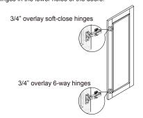
**Step 7:** Connect the doors to the box, hinges on the door panels snap into the hinges on the side
