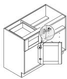
**Step 8:** Install the shelf supports at the desired height then place shelves on top of the supports. Adjust the hinges to ensure that the clearance for all doors is the same. Finally, check the firmness and stability of the cabinet tightening the cam locks as necessary.
